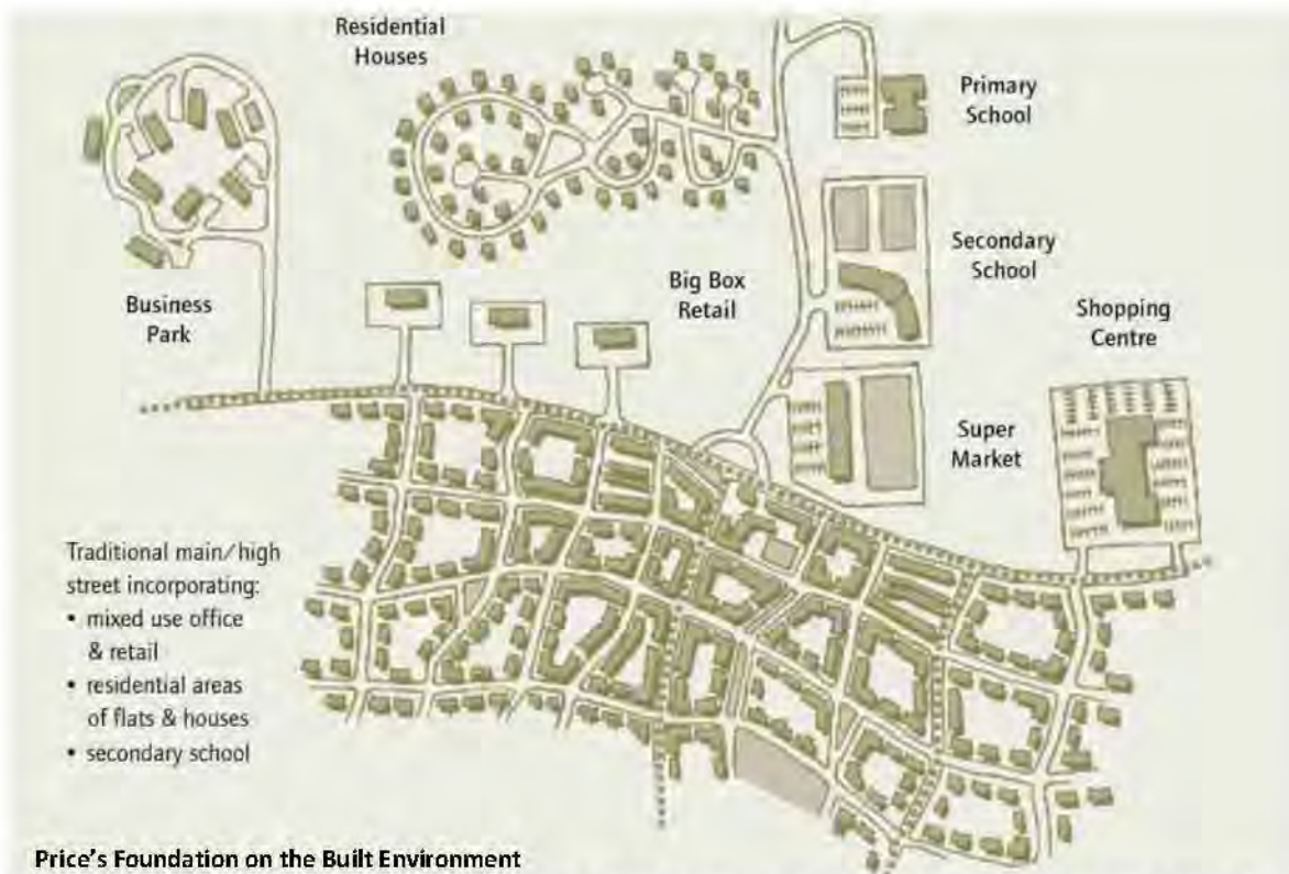
Price's Foundation on the Built Environment Inefficient land use patterns (sprawl) are shown on the top half of the above graphic, while efficient land use patterns (traditional) are shown on the bottom half.
