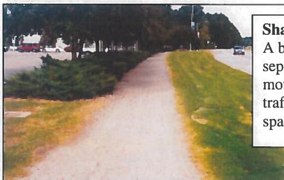
**Shared Use Path**—A bikeway physically separated from motorized vehicular traffic by an open space or barrier.
